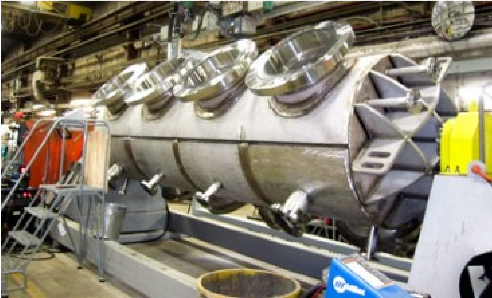
Final stages of the build of a commercial four-core FT reactor
